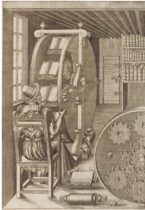
Figure 7. Bookwheel, a mechanical reader designed by Agostino Ramelli from his book Le diverse et artificiose machine , 1588.
